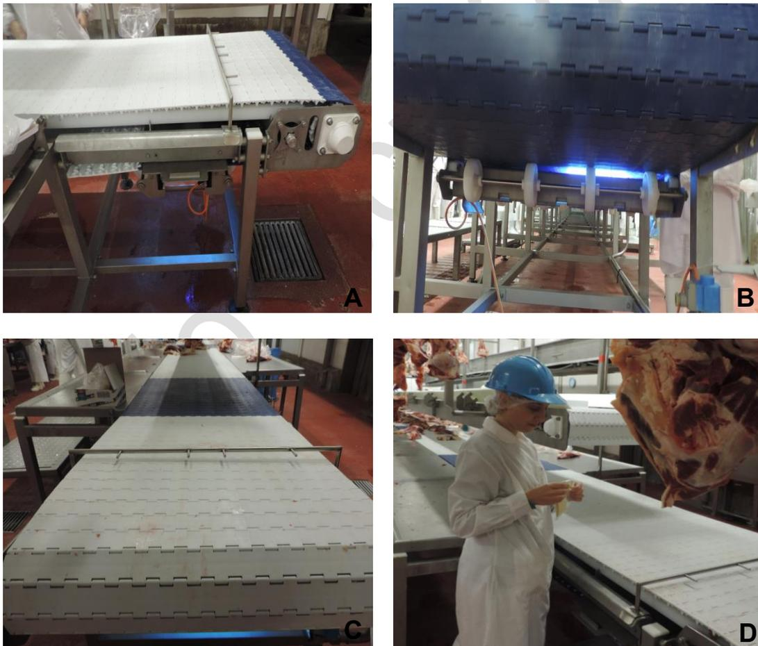
**Fig. 1.** A) Position of the UV-C germicidal emitting lamps. B) Picture shows the areas directly exposed and non-exposed to the UV-C light. C, D) Frame and sampling place along the production line.
