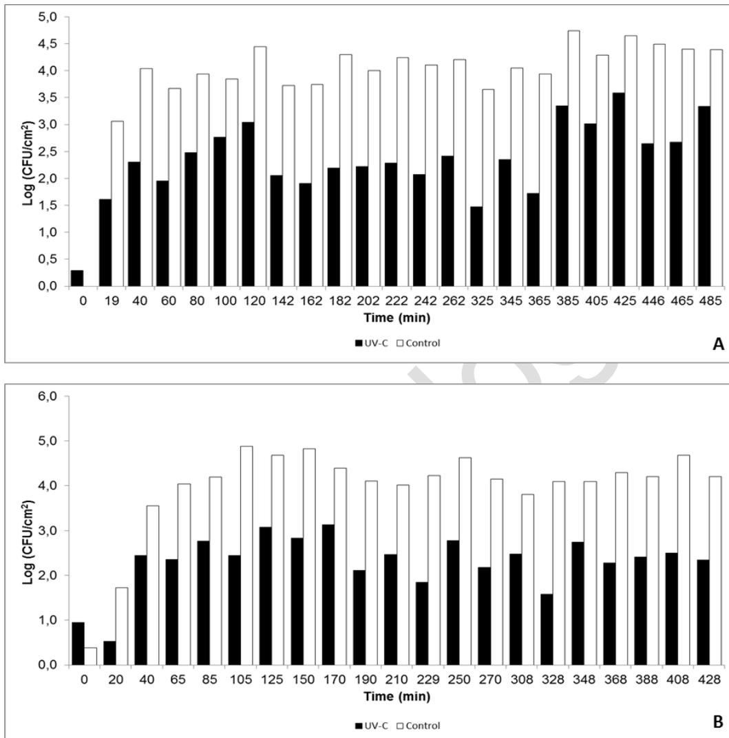
**Fig. 3.** Effect of UV-C irradiation on the APC expressed as Log (CFU/cm<sup>2</sup>) over time. A, samples collected on day 2; B samples collected on day 3. Control, non UV-C exposed samples; UV-C, UV-C exposed samples.
