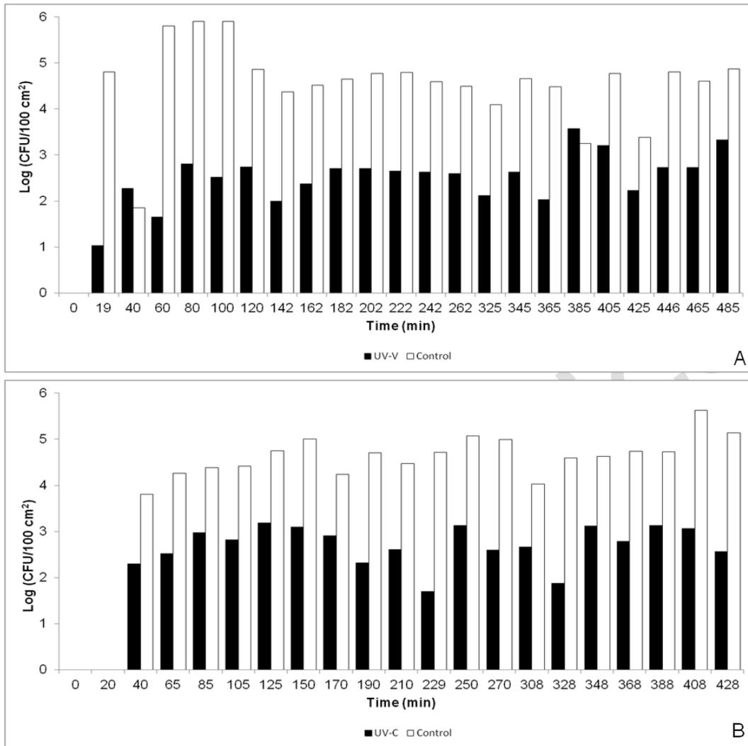
**Fig. 4.** Effect of UV-C irradiation on coliform bacteria CB expressed as Log (CFU/100 cm<sup>2</sup>) over time. A, samples collected on day 2; B samples collected on day 3. Control, non UV-C exposed samples; UV-C, UV-C exposed samples.
