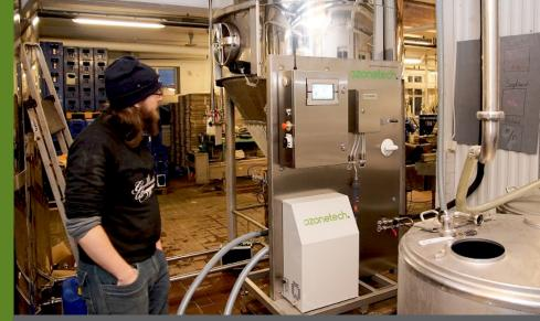
The RENA Vivo A-series system is connected to tanks and other process equipment during <u>CIP sanitation</u>. The brewmaster Johan Hansson is observing the system during operation.
